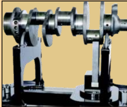
Design allows ram to be positioned directly under #1 rod journal
