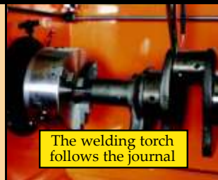
The crankshaft turns on its centerline
